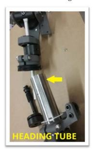
6. Loosen the nut for #88 Worm Box Stud
